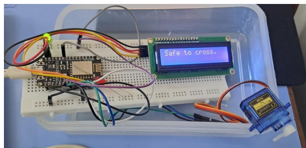
Fig. 13. Fifteen seconds after the train passes, the motor reopens the interface.
